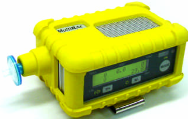
Figure 18 Compact, multi-sensor confined space gas detector with LEL, O 2 , CO, H 2 S and PID equipped with 10.6 eV lamp. (Courtesy of RAE Systems Inc. Sunnyvale, CA)
