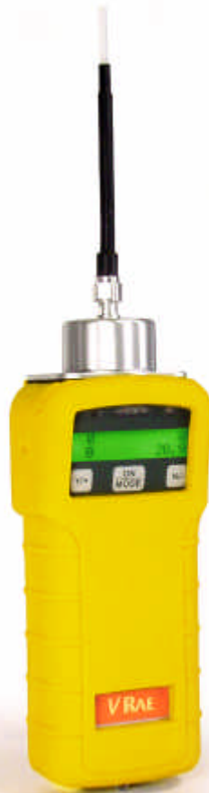
Figure 8. 1-5 Sensor VRAE Gas Detector equipped with dual-mode combustible sensor capable of both catalytic oxidation (0 – 100% LEL) and thermal conductivity (0 – 100% volume) detection. (Courtesy RAE Systems Inc., Sunnyvale, CA)
