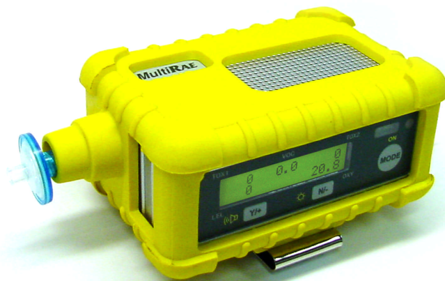
Figure 1. MultiRAE Plus Multi-Gas Monitor with PID
